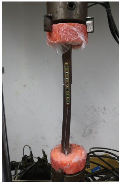
Figure 6: The torsion test on an MTS 858
