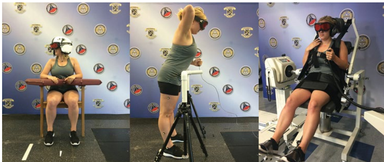
Figure 1: Proprioception testing (Cervical JPS, Trunk JPS, and Trunk TTDPM).
