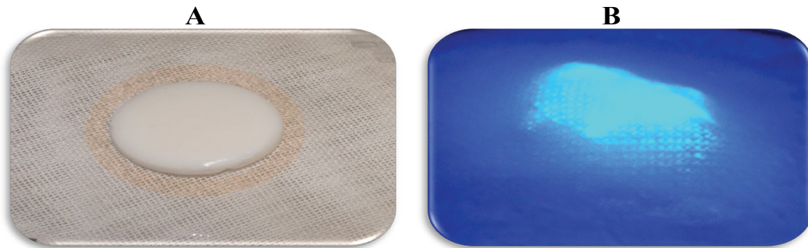
Figure 5: Depiction of nanocellulose aerogel peptide conjugates biosensor (diameter of 2.1 cm) with fluorescent protease activation interfaced in a multilayer bandage prototype with and without ultraviolet illumination. Image A demonstrates a gauze contact layer, barrier layer, and biosensor layer without ultraviolet activation. Image B depicts a barrier layer and gauze top layer above the biosensor layer with ultraviolet illumination.
