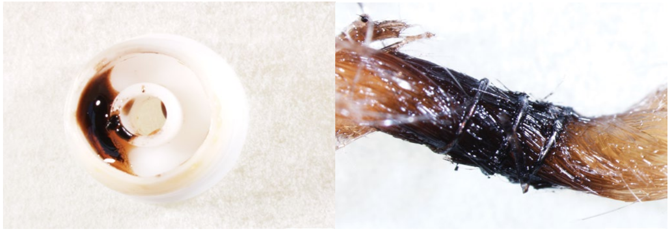
Figure 1: Electronic cigarette mouthpiece with particles of insoluble apparently thermally decomposed tobacco extract from the aerosol (left); and evidence of thermally decomposed material on the wick in proximity to the heating element (right).
