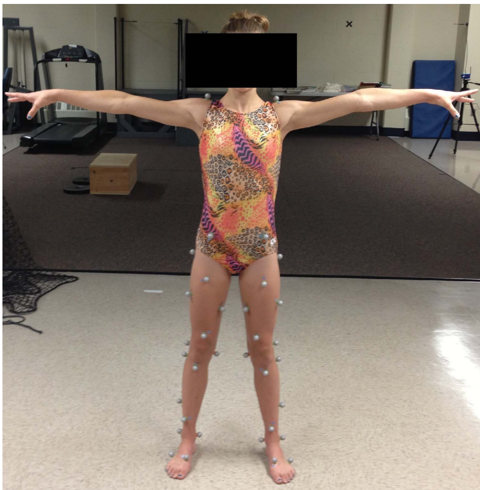
Figure 3: Lower extremity MOCAP tracking marker configuration
